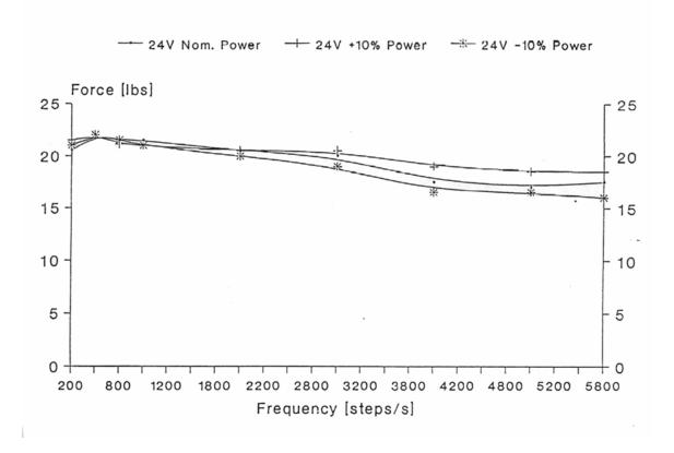
Figure 10. XL 3000 High Resolution Pump Typical Plunger Force Curve (Dynamic Force)
