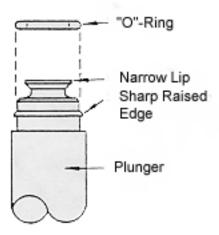
*Caution:* 5.0 mL, 10.0 mL and 25.0 mL syringes have "O"-rings beneath the seal. Be careful not to damage the "O"-ring. If it is necessary to replace the "O"-ring, simply slip the new "O"-ring over the narrow lip on the plunger. It may be necessary to use needle nose pliers to assist in removing the "O"-ring from the 10.0 mL and 25.0 mL plunger.
